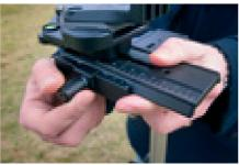
FIND THE CENTRE POINT. Adjust the first plate that moves the camera leftto-right so that the centre of the lens sits directly over the centre of the tripod. Some heads will allow you to point the camera down at the head to align it through the viewfinder.
