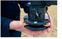
**START MOUNT CAMERA AND LEVEL** TRIPOD. Lock off all adjustments on the tripod and ensure the head is securely on. Place the camera on the tripod in a portrait position and, using the spirit level, adjust the legs or levelling plate to get it spot on.
