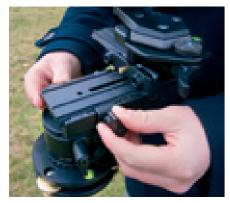
NODAL POSITION (FRONT-TO-BACK). Now adjust the second slider, moving the camera forwards and backwards, so that the lens sits over the centre of the tripod. The exact point can be anywhere between the front of the lens and the sensor, so it's a matter of trial and error.
